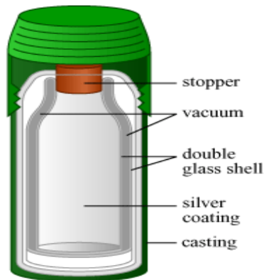
Fig.6 Internal structure of a vacuum flask.
