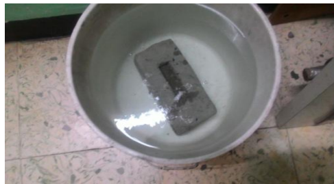
Fig.6:water absorption test
