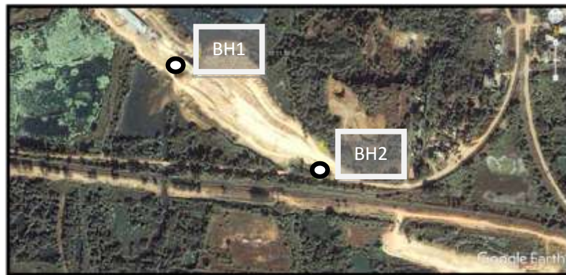
Fig 4.1 Borehole Location Map
