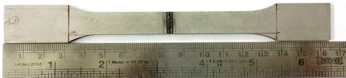
Figure-6. Specimen for tensile test
