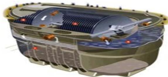
The variables in the rotating biological contactors were hydraulic retention time, disc submergence level in the wastewater, rotation speeds, pH control, supplementary nutrients and volumetric flow rate of the wastewater. The influent was taken at volumetric flow rate of 30, 36, 45 and 60 l/day. The samples were taken for analysis for each volumetric flow rate after two times of corresponding retention time, based on steady state assumption
