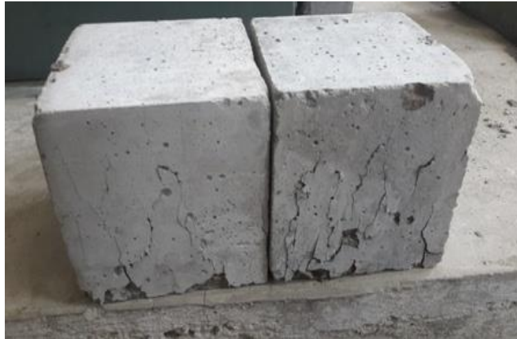
Fig -1: Crack Developed After Casting Of Cubes
