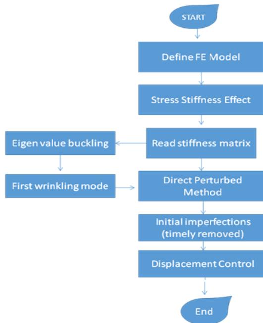
**Fig 3. Flowchart of wrinkling computation**
