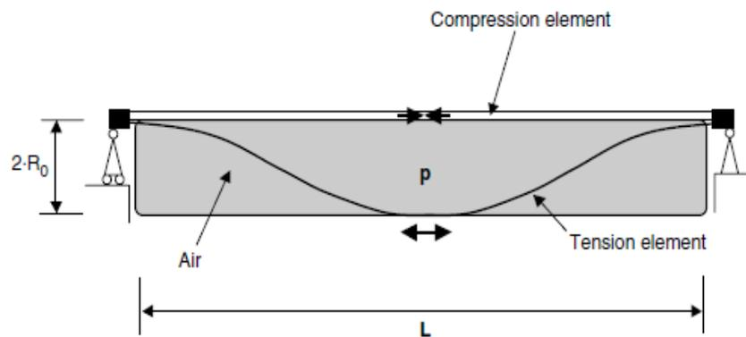
**Fig 1. Representation of cylindrical shaped Tensairity beam**
