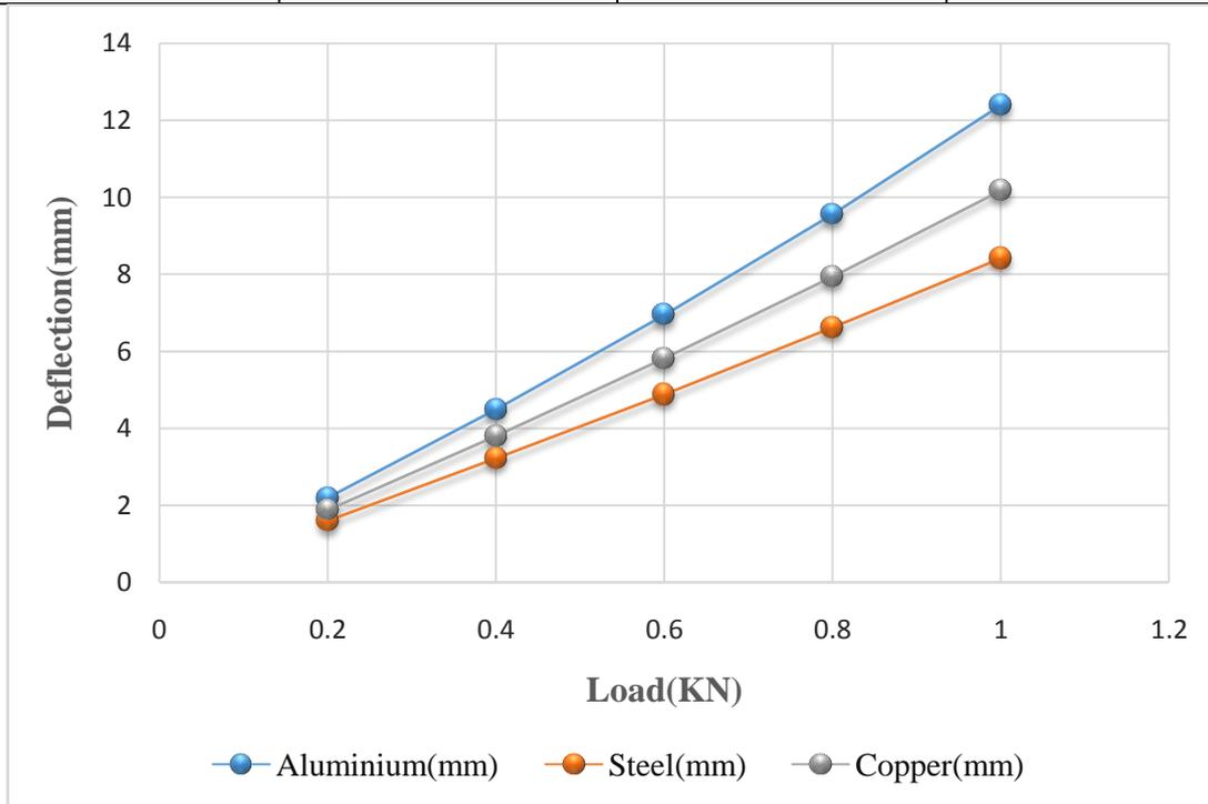
**Fig 8 Load-Displacement response graph for different chord materials**
