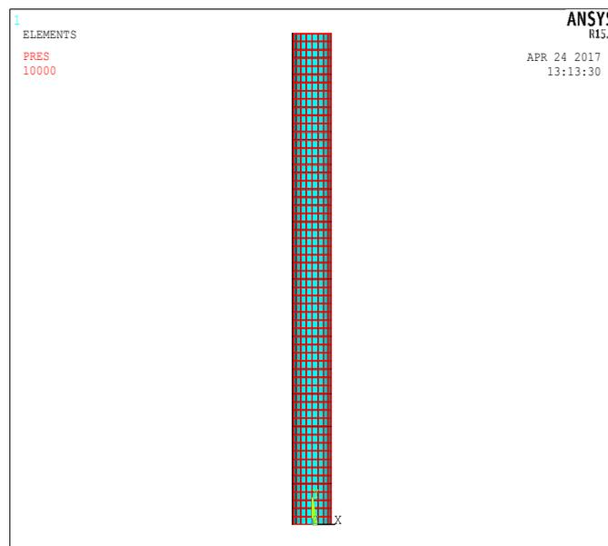
Fig 7. Meshed model of inflatable beam
