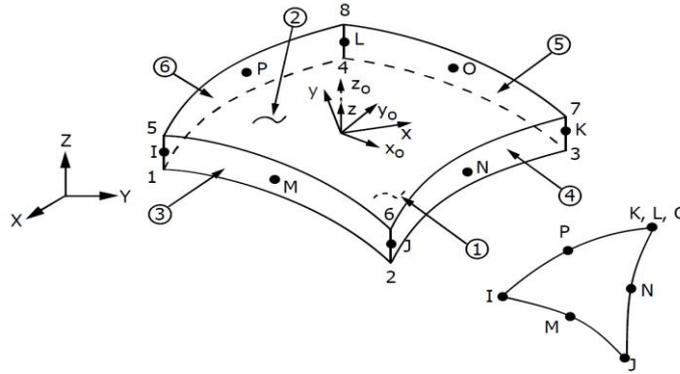
Fig 5.Configurations of shell 281 element
