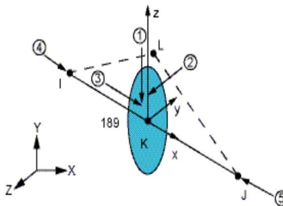
Fig 6.Configurations of beam189 element
