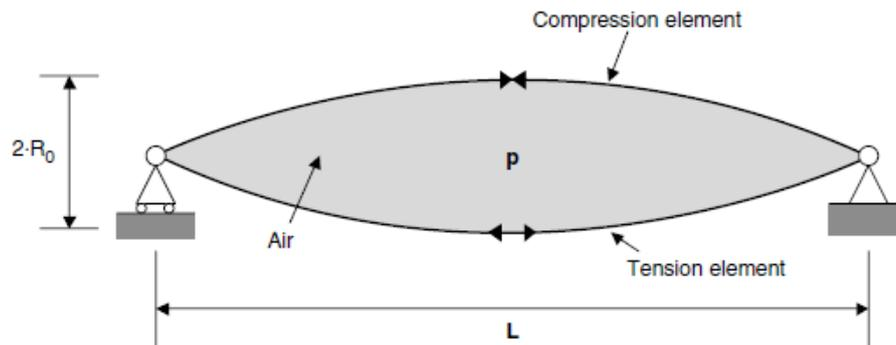
**Fig 2. Representation of spindle shape Tensairity beam**
