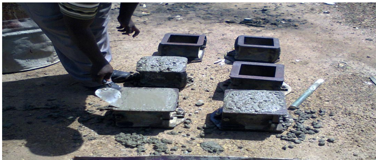
Fig. 2.1 Filling the cubes of size 150X150X150 (mm) with concrete
