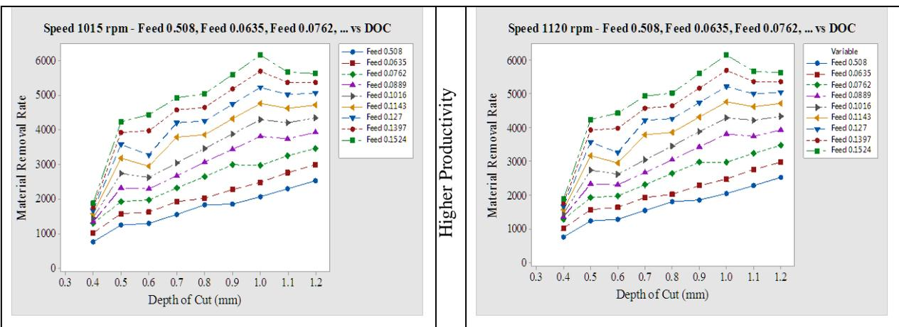
Fig. 4.5 Speed 1015, 1120 (rpm) – Feed 0.0508, 0.0635, 0.0762 .....0.1524 (mm / rev) Vs Depth of cut (mm)
