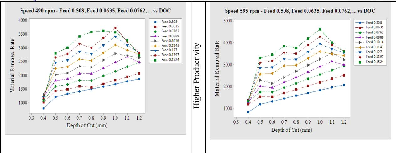
Fig. 4.3 Speed 490, 595 (rpm) – Feed 0.0508, 0.0635, 0.0762 .....0.1524 (mm / rev) Vs Depth of cut (mm)
