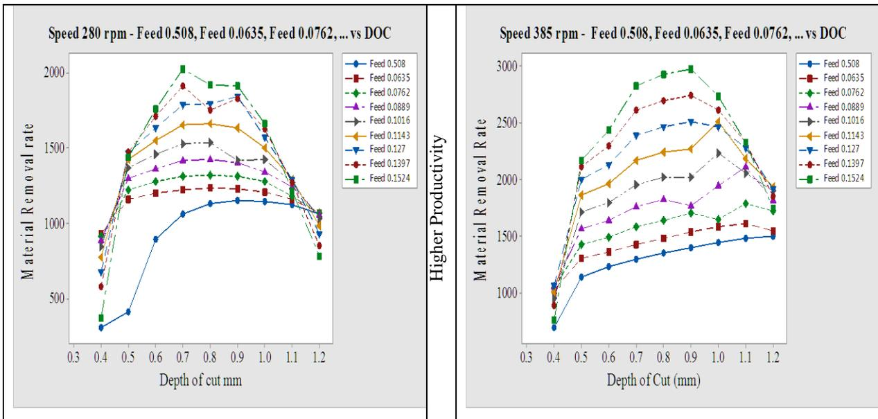
Fig. 4.2 Speed 280, 385 (rpm) – Feed 0.0508, 0.0635, 0.0762 .....0.1524 (mm / rev) Vs Depth of cut (mm)
