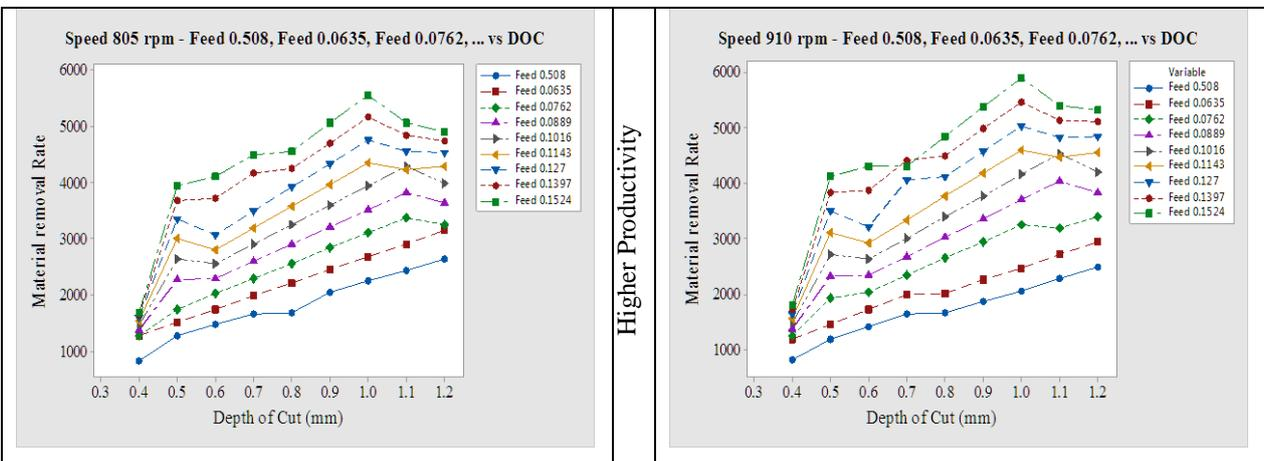
Fig. 4.4 Speed 805, 910 (rpm) – Feed 0.0508, 0.0635, 0.0762 .....0.1524 (mm / rev) Vs Depth of cut (mm)
