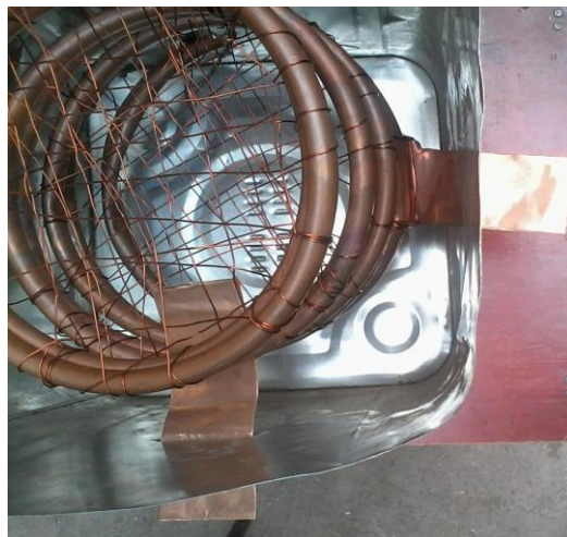
Fig.9 Copper plate installed for Thermoelectric Module
