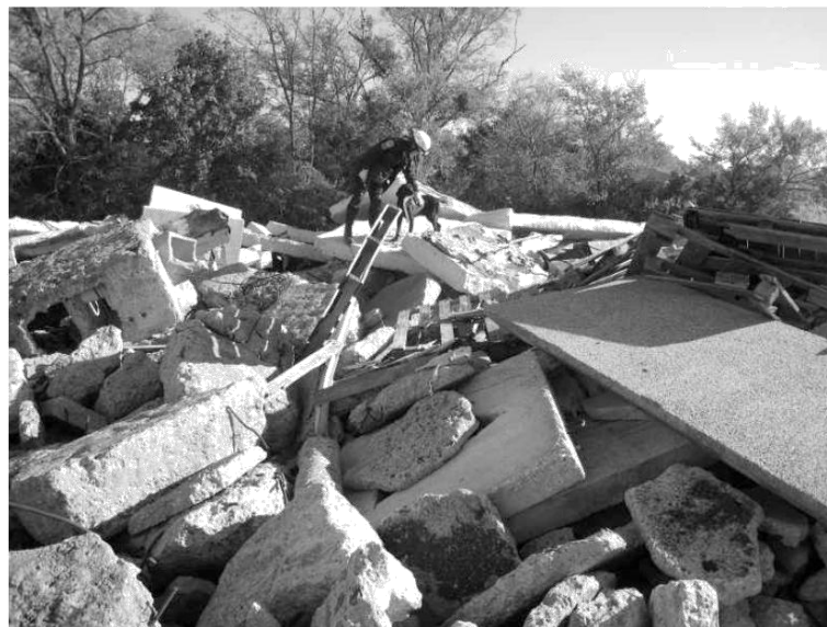
Figure 1. Handler rewards an USAR dog after the successful wireless activation of a drop bag. Testing indicated that the network's signal strength went from 100% to 0% 2.5 ft into any of the many holes that can be seen on the pile. Handler and dog TF1 (TX).
