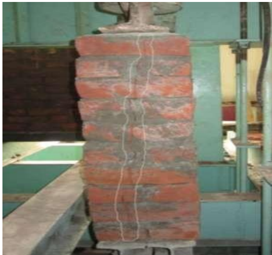
Fig.7 Crack in brick wall
