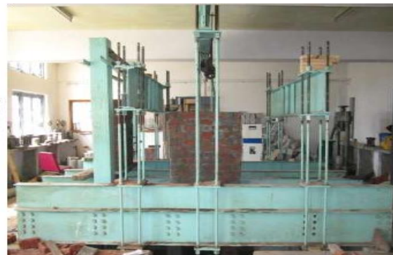
Fig.2 Brick wall constructed on loading frame
