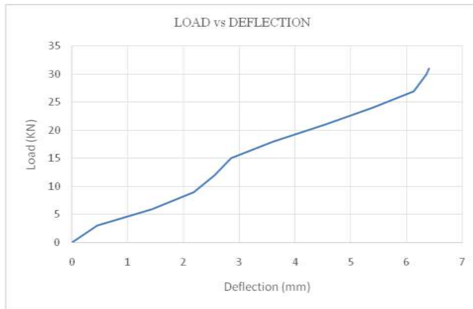
Fig 4.8 Load deflection graph v/s for HCWOS beam specimen 3
