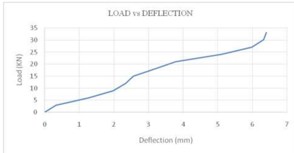
Fig 4.6 Load v/s deflection graph for HCWOS beam specimen 1
