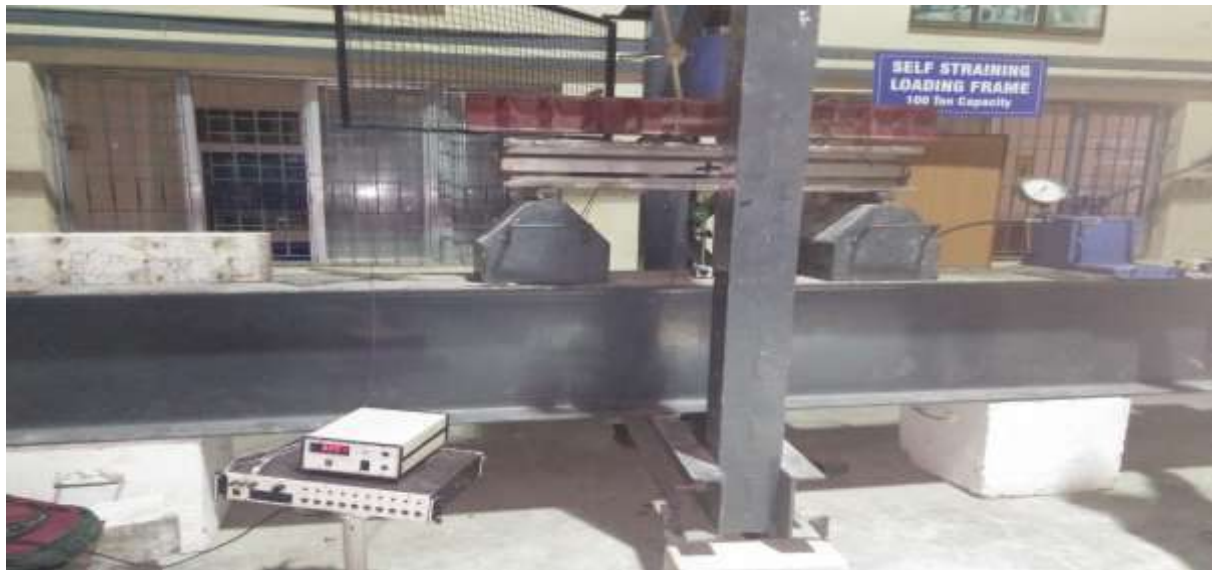
Fig4.2 Experimental set-up for the test specimens
