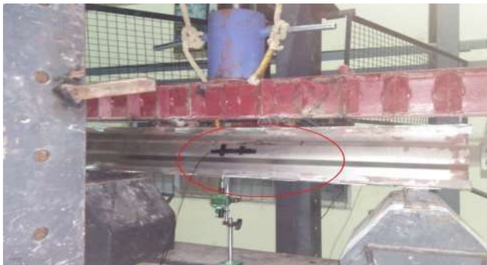
Fig4.3 Failure of HCWOS beam
