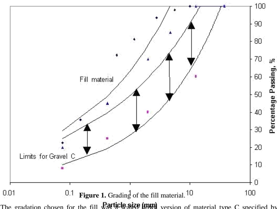
The gradation chosen for the fill was a scaled down version of material type C specified by the Malaysian Federal Works Department, (1988). The fill material was scaled down using a scale of 1:4 in order to account for the modeling requirements. Figure 1 details the gradation limits for material C and the gradation for the scaled fill material.
