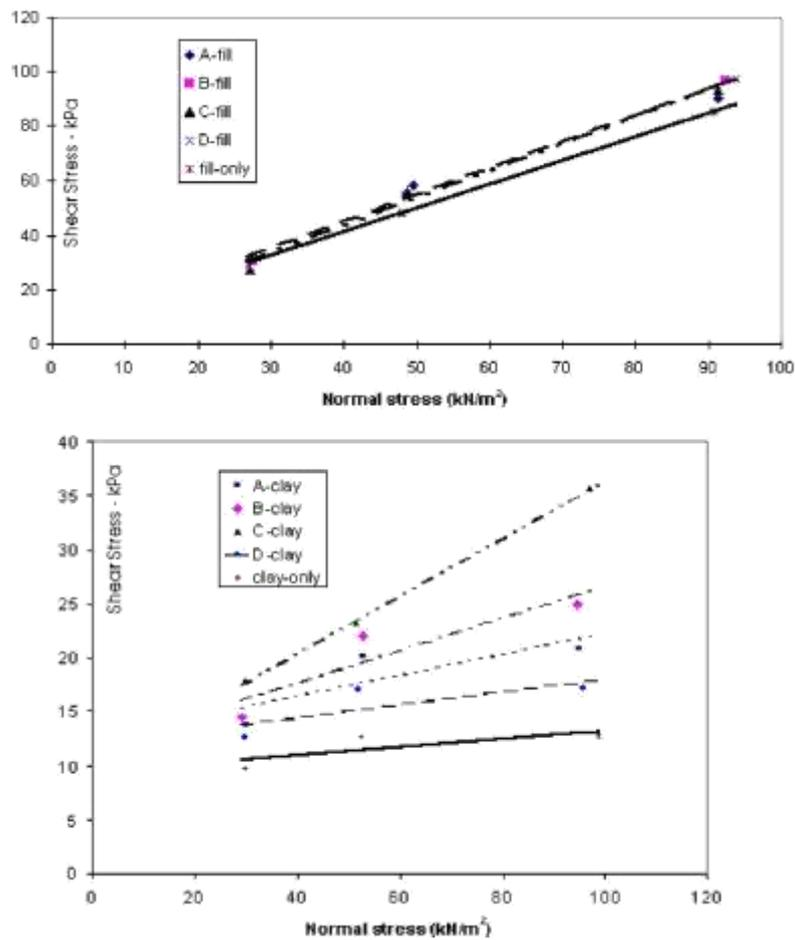
**Figure 4.** Failure envelopes of the soil/geotextile interfaces.
