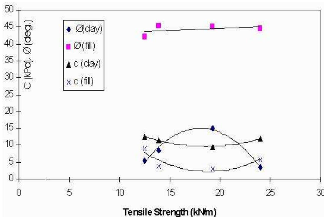
**Figure 5.** Shear strength versus tensile strength for the soil/geotextile interfaces.
