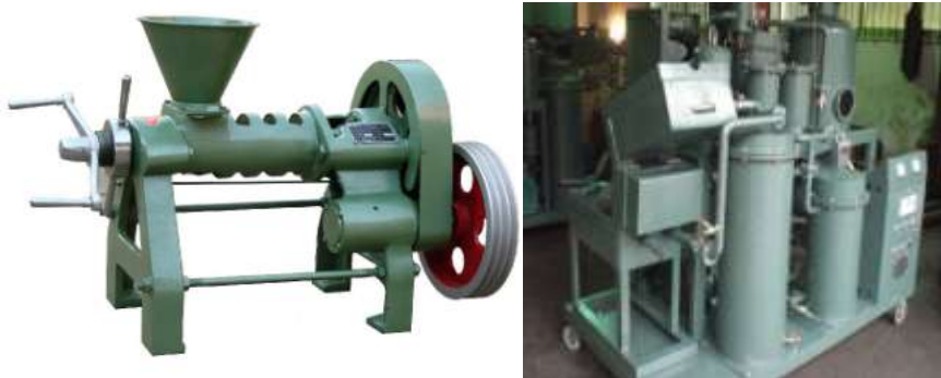
Fig.6 (a) Small jatropha oil extraction machinery being used in India (b) Crude-jatropha-oil filtering systems
