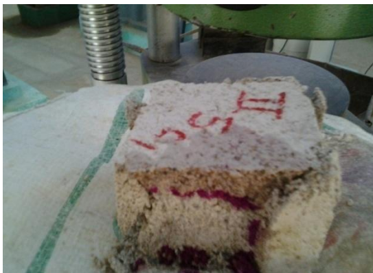
Fig.3 After compressive strength test, cubes sprayed with phenolphthalein indicator to know depth of carbonation. Depth of carbonation not measured.
