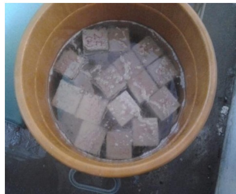
Fig. 4 Durability test on cube samples with 2% H 2 SO 4 Solution
