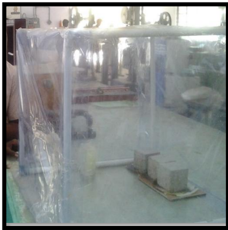
Fig. 1 CO 2 Chamber for accelerated curing
