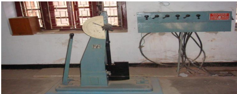
Fig 2.7 Charpy impact tester for toughness test
