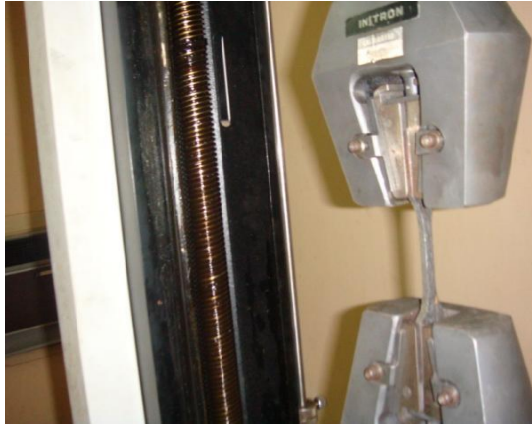
Fig. 2.8 Instron 1195 machine for tensile test
