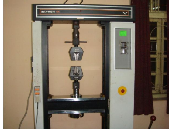
Fig. 2.8 Instron 1195 machine for tensile test
