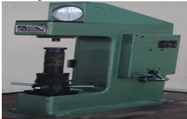
Fig. 2.4 Rockwell hardness testing machine
