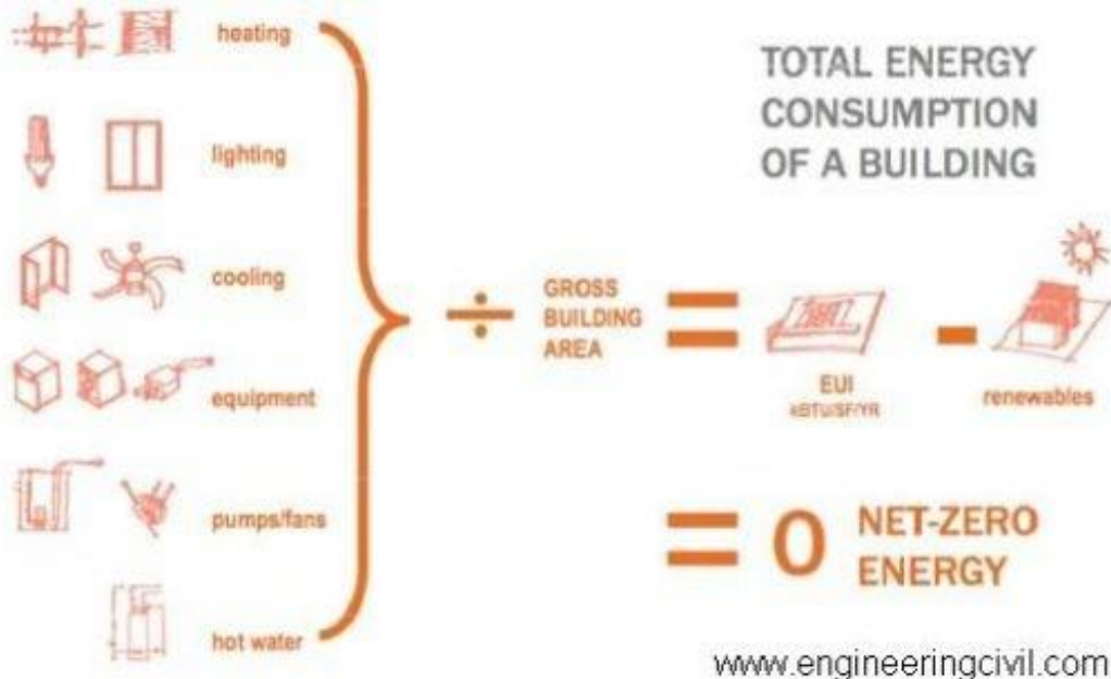
(Figure 1.3: Total Energy Consumption Equation)
