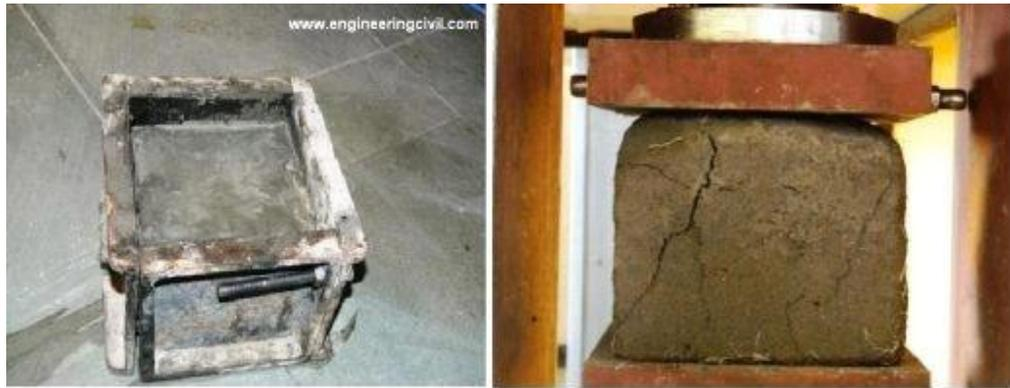
The sample was then tested in compressive strength testing machine as shown above and below.
