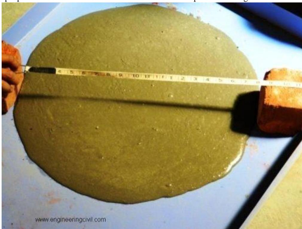
Concrete is filled in the mould in two layers, each layer is tamped 25 times & then after removal of the mould, the table on which mould is kept is raised & dropped for 15
