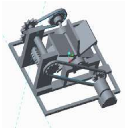
Fig.3. Front View of the de-husker
