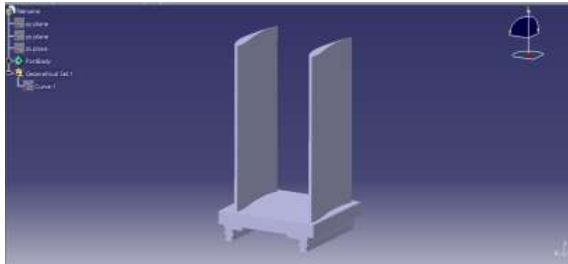
Fig.4: Case-2: Turbine Blade with Flat Damper
