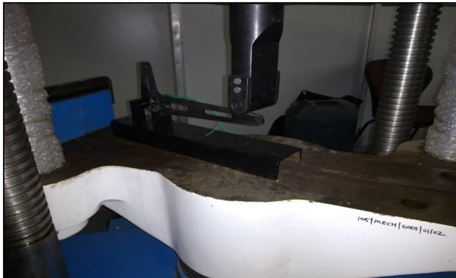
Figure 5: Testing of optimized bell crank lever on UTM
