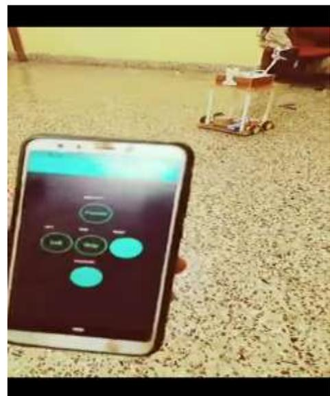
Fig 4: Above image shows blynk app screen with widgets to control the wheeled robot
