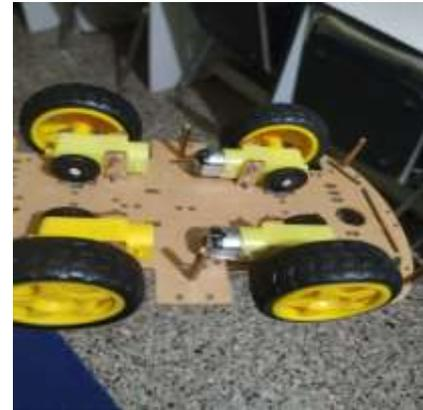
Fig2. Interfacing BO motors with chassis
