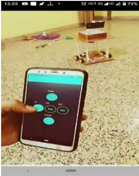
**Fig5. The smart phone loaded with droid cam app streams the current situation of the ward by means of video streaming that could be seen at remote server**
