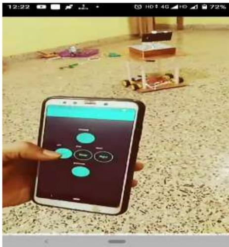
**Fig6. The direction of the robot can be controlled using widgets( Buttons ) present in blynk app, based on the instructions it changes its direction of the movement.**
