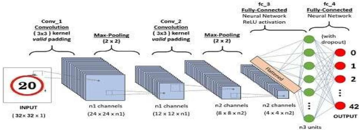
Fig.4.CNN model architecture
