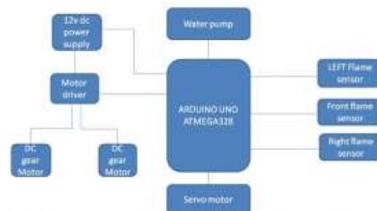
Fig: V(a) Purposed block diagram of Fire Fighting Robot.
