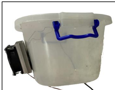
Fig 3. Side View of Water Cooling System
