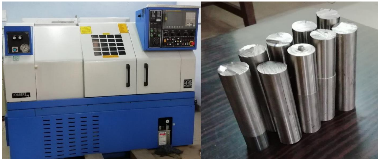
Figure 1: a) JOBBER LM, CNC Machine from ACE designer b) 316 L samples after turning operation.
