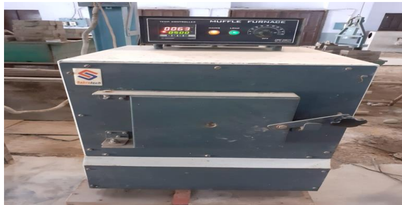
Fig. 1. Muffle Furnace for Sintering.
