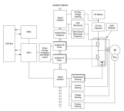
Fig. 7 EV Inverter Block Diagram [5]
