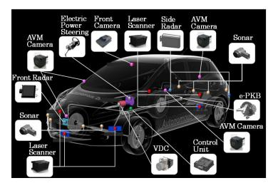
Fig. 9. Key devices for autonomous driving
