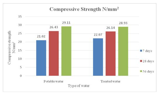
Fig 4.2 - Compressive Strength of PW& TWW Concrete Cube Specimens
