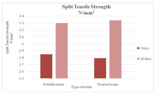
Fig 4.4 - Split Tensile Strength of PW& TWW
