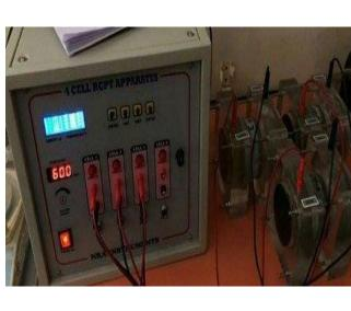
Fig 4.5 - Test Setup for RCPT
