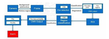
regions into a complete region. In this way, the whole moving object is detected. In the fire detection approach, we will calculate the size of white regions in system can capture the moving The whole frame. method will set a threshold and if the size of moving objects exceeds the threshold, the next detection steps will be implemented.
