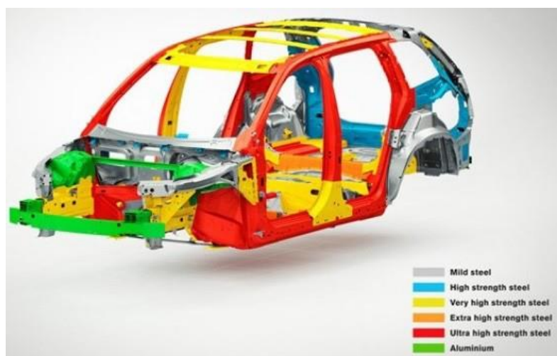
Figure 3. The materials used in new XC90 (Courtesy of Volvo Car Corporation)
