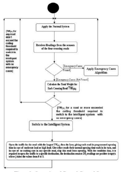
Figure 3: Operation of Central Control System
