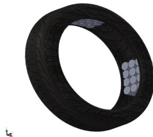
FIG 1- Layout of arrangement of piezo discs in the tyre
