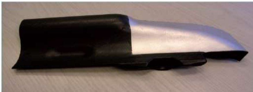
Fig 2.4.1 Heat Shield Made of Composite
