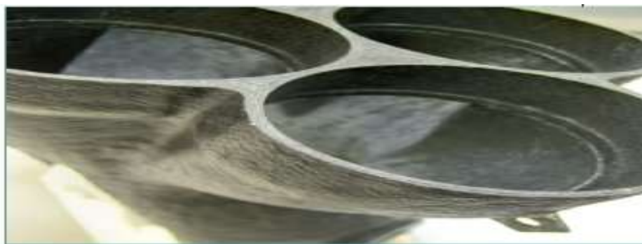
Fig 2.3.1 Motorsport Duct Made of Composite Material
