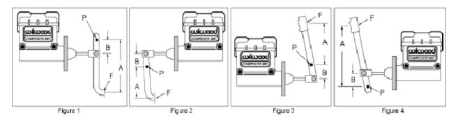
A = Distance from pivot point to middle of push / pull point
