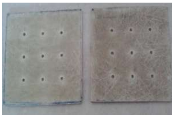
Fig.7 View Of Entrance Side Of Drilled Holes For Different Cutting Parameters By Both drills
