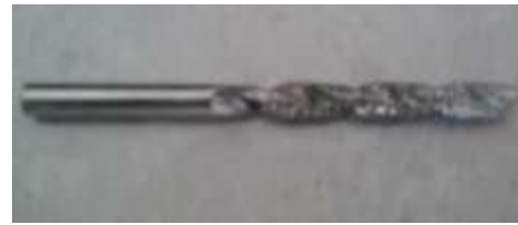
Fig.5 Diamond coated HSS twist bit
