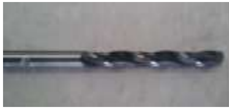
Fig.4 Uncoated HSS twist bit
