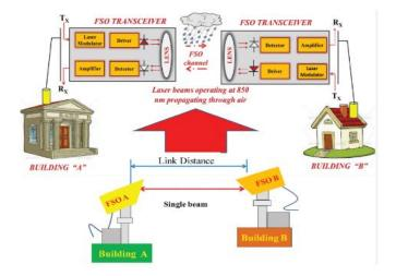
Fig. 2. Components of FSO System
