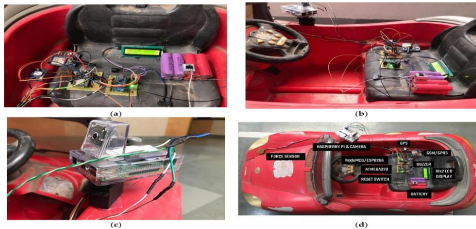
Fig 4: Installation of developed IoT kit on a car. (a) Car with IoT Sensor and LED Display, (b) Car with IoT Sensor, (c) Car with IoT Kit with Camera, (d) Car with labeling of each Device in IoT Development kit
