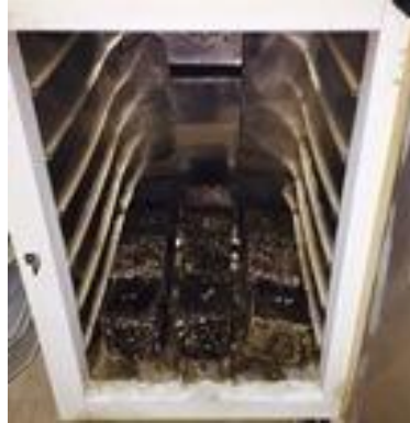
Fig: 6. Curing of specimens
