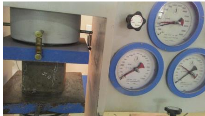
Fig.8. Testing Compressive Strength
