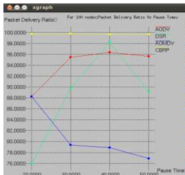
Fig 12: Packet Delivery Ratio Against Different Pause Time
