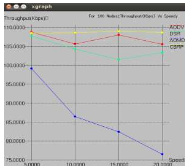
Fig 9: Throughput Against Different Speeds of the Nodes
