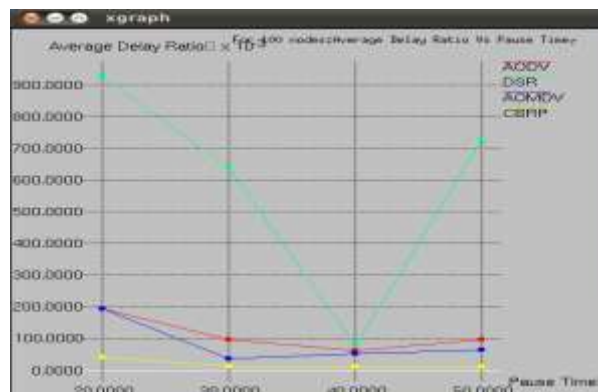
Fig 8: Average Delay Against Different Pause Time
