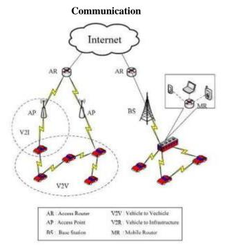
Fig 2: General Model of Vehicular Networks
