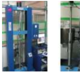
Fig. 1.4: Computer controlled Testing machine with the extrusion process fixtures
