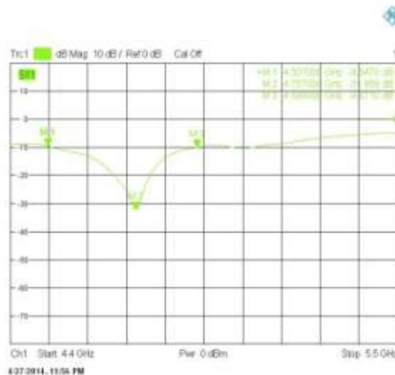
Figure12. S parameter Display of fabricated slot antenna
