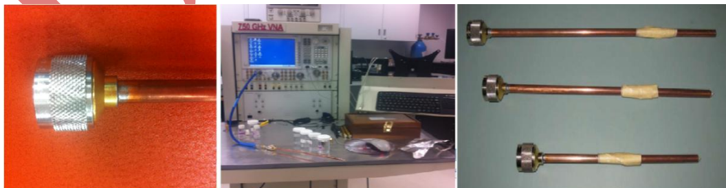
Fig 4: Handmade probes, network analyzer and connector
