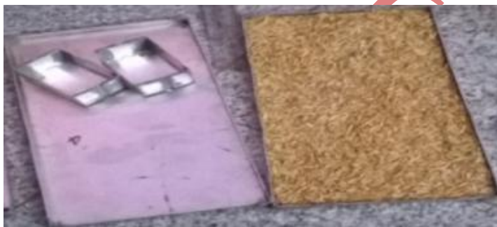
Fig no 2.2.1 mould used for fabrication of composites and cured cut samples.
