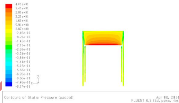
Fig9: Pressure contours for 30° inclination
