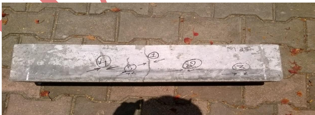
Fig 7: Cracking Pattern for the M 25 Grade Concrete
