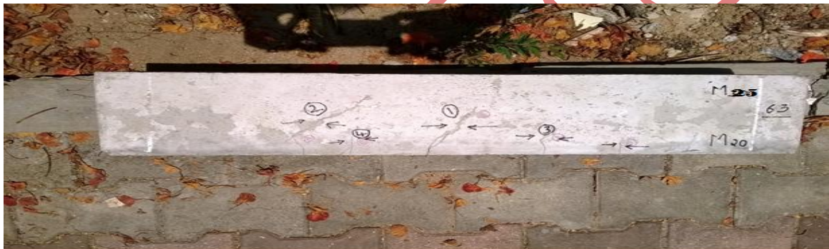
Fig 9: Cracking Pattern for the M_{20}+M_{25} @ 63 Mm
