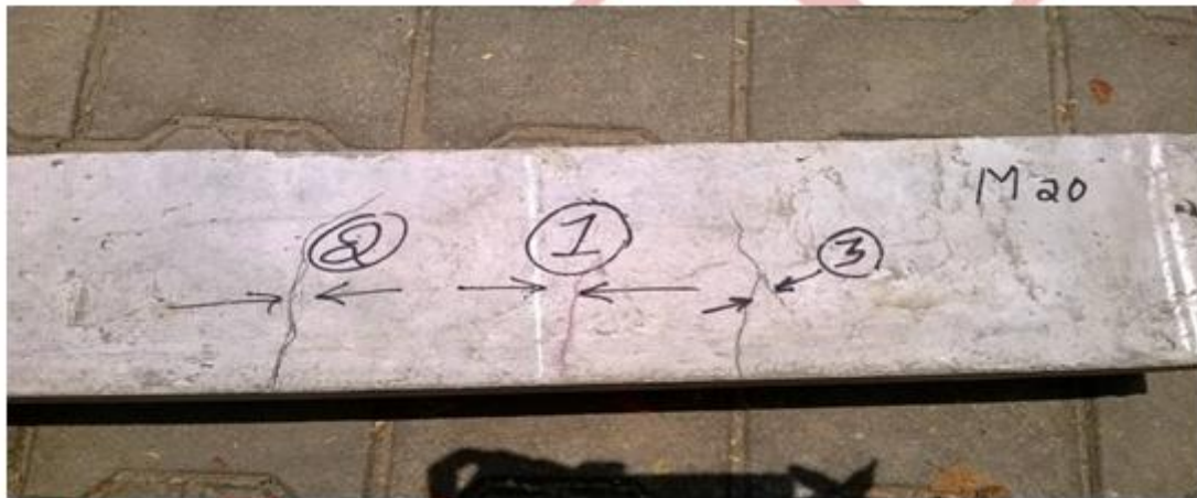
Fig 6: Cracking Pattern for the M 20 Grade Concrete
