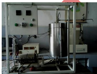
Figure 3 Photo of Bio-ethanol steam reforming laboratory plant.
