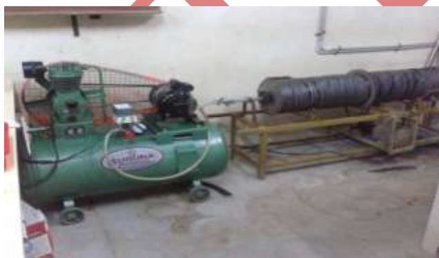
Fig. 1 Laboratory scale rotary drum with compressor
